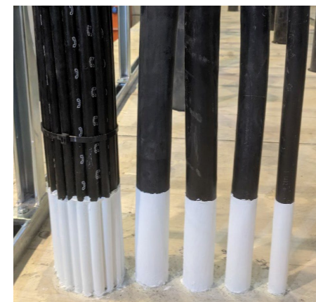
Typical sample of penetrating services with annular gap widths between 10 and 30mm
